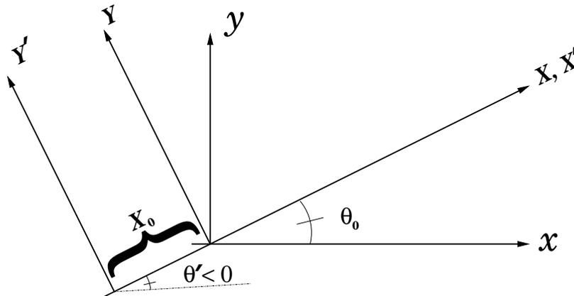
FIGURE 6. Graphical definition of the rotated and shifted coordinate system (the primed coordinate system) in terms of the original coordinate system used in Figure 4. The length scale changes between the lower and upper case coordinate systems by a factor of  $\beta/\varepsilon$ ; so for example  $R = r\beta/\varepsilon$ .
