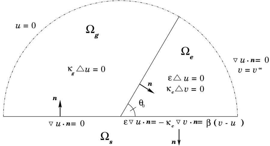
FIGURE 4. Domain  $\Omega := \Omega_g \cup \Omega_e$ , along with the differential equations and boundary conditions. Note the orientation of the unit vectors at the interfaces.  $0 < \theta_0 < \pi/2$ . The dependent variables  $u$  and  $v$  are the component potentials associated with the oxidants and the current.
