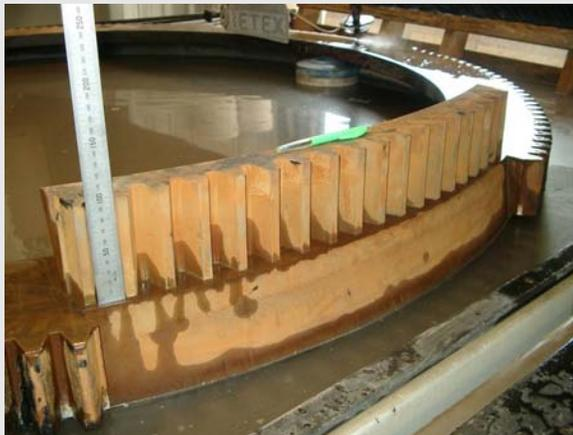
10-cm thick wind turbine gear
