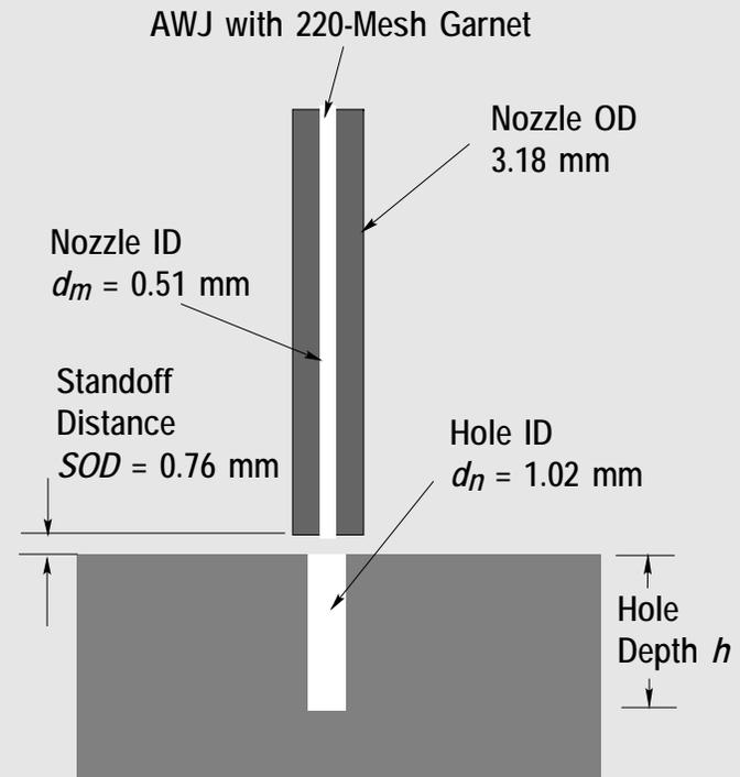
**Configurations for CFD modeling of hole drilling**
