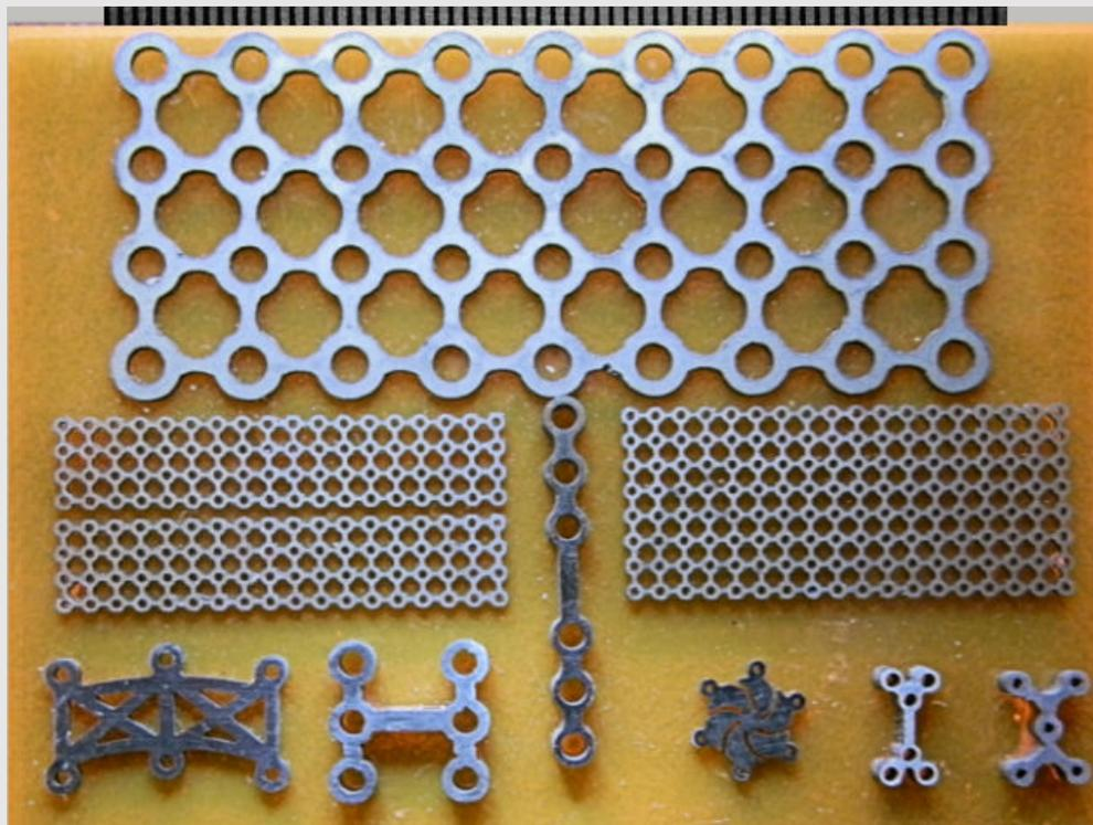
AWJ-machined micro-plates and Mini-plates (titanium and stainless steel)
