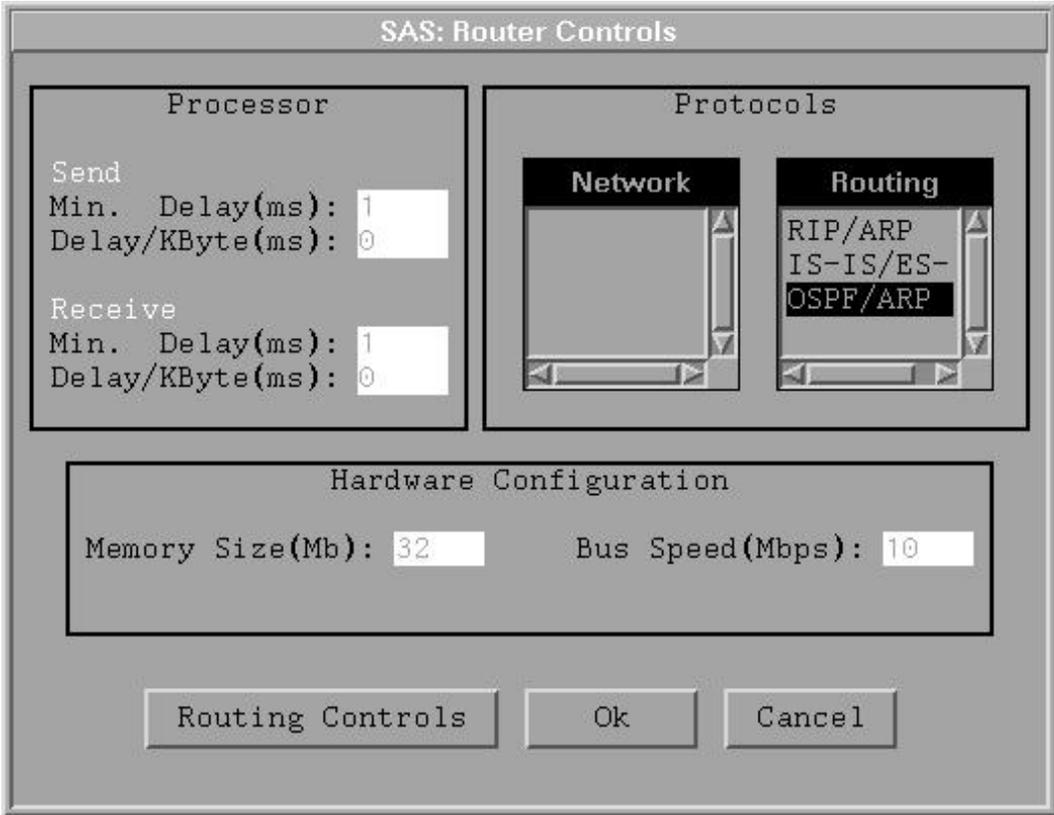
Figure 4.14. Sample Router Model Controls
